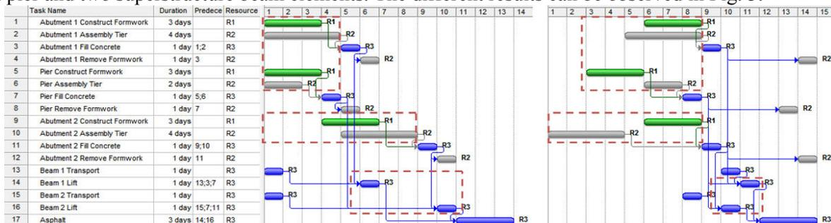
Fig. 3: Different results of the forward (left) and backward simulation (right) without dependencies (colours: resources, arrows: precedence constraints, dashed boxes: changed order/earlier start).
