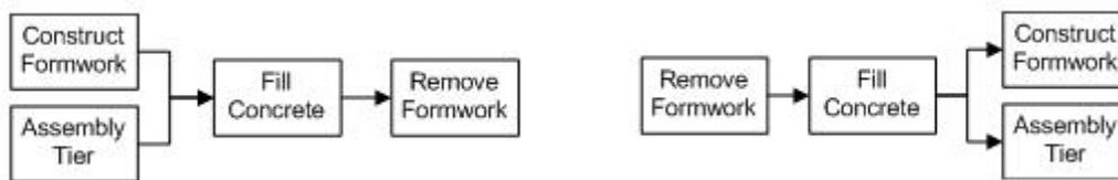
Fig. 2: Precedence relationships for forward simulation (left) and for backward simulation (right).
