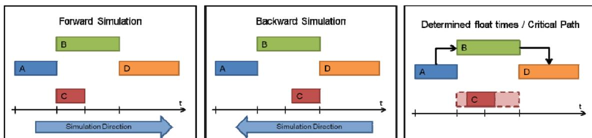
Figure 1: Concept of determining float time and critical path combining forward (left) and backward simulation (middle).
