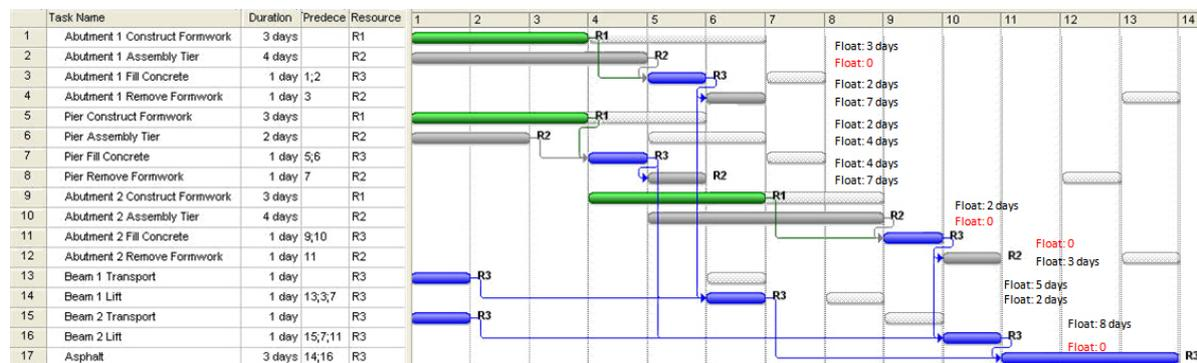
Fig. 5: Results of the communicating simulations: Float times (backward simulation results transparent grey)
