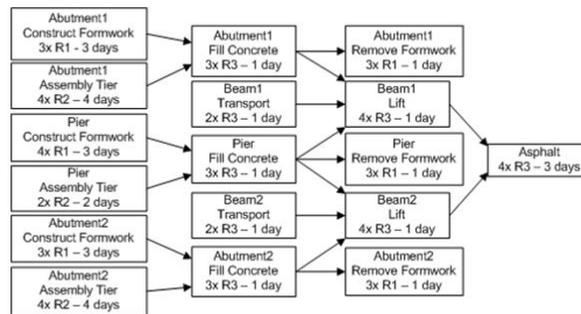
Fig. 4: Task structure of the example project.
