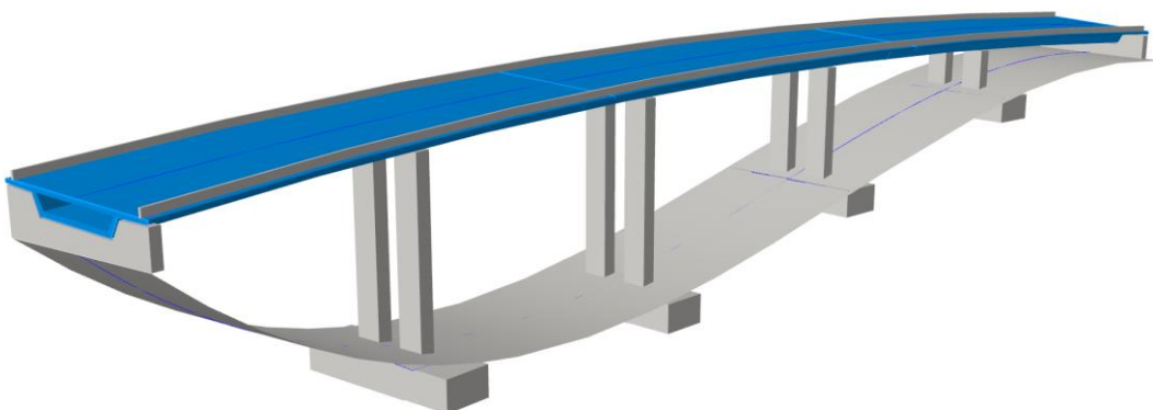
Figure 7: Bridge BIM model generated by the KBE prototype, version 1
