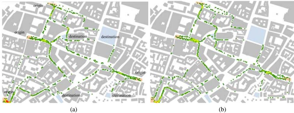
Figure 13: (a) Screenshot of a simulation using a static field. (b) Screenshot of a simulation using a dynamic navigation field in combination with the navigation graph.
