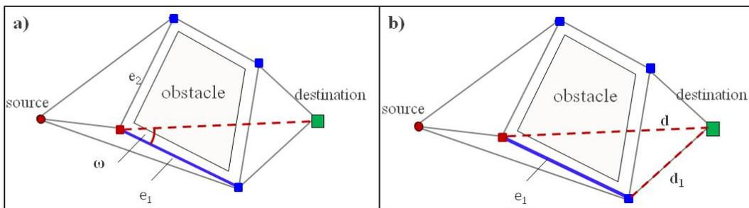
Fig. 3 a) angle derivation  $\omega$  of edge  $e_1$  b) relative distance enhancement of edge  $e_1$ :  $d_1/d$
