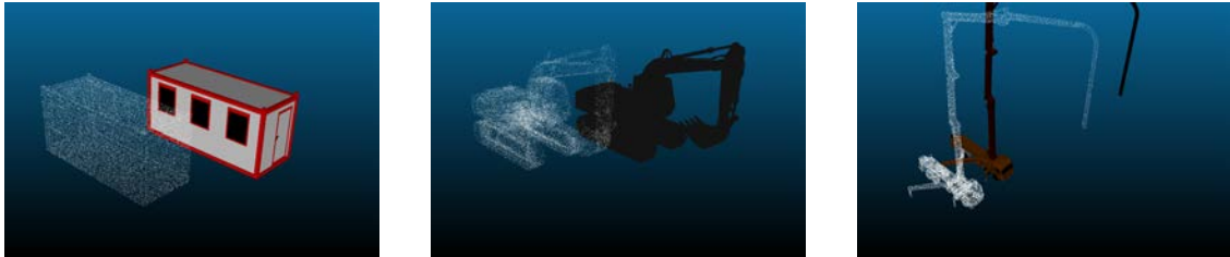
Figure 5.3: STL examples and their point cloud representation (container,excavator,concrete pump)
